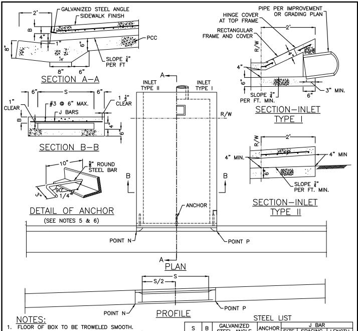
2. WHEN THE TOE OF SLOPE IS WITHIN THE R/W INLET TYPE I BEGINS AT THE TOE RATHER THAN AT THE R/W LINE.
