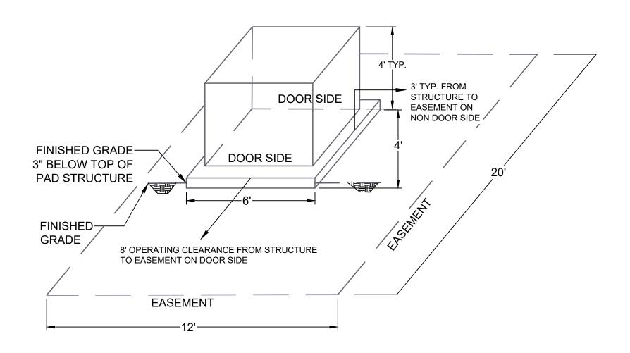
NOTE: 4-Foot clearance is required from edge of pad for automation.
