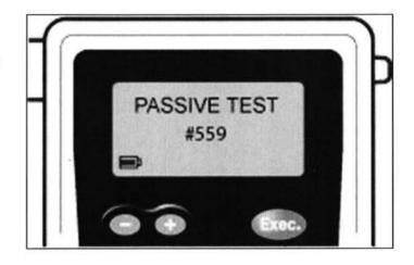
A passive test will etermine only the presence of alcohol and gives no measurement of the amount of alcohol in a sample
